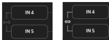
Figure 21: DSP Page – Linking Analog Audio Ports
