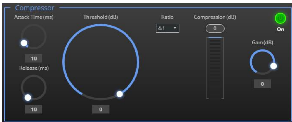
Figure 30: Processing View – Compressor Module
