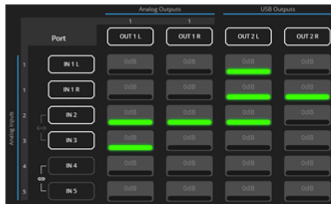
Figure 39: Matrix Page – Multiple Input-Output Cross-Points
