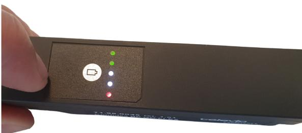
A total of five LEDs are representing the remaining capacity, each representing 20% charge.
