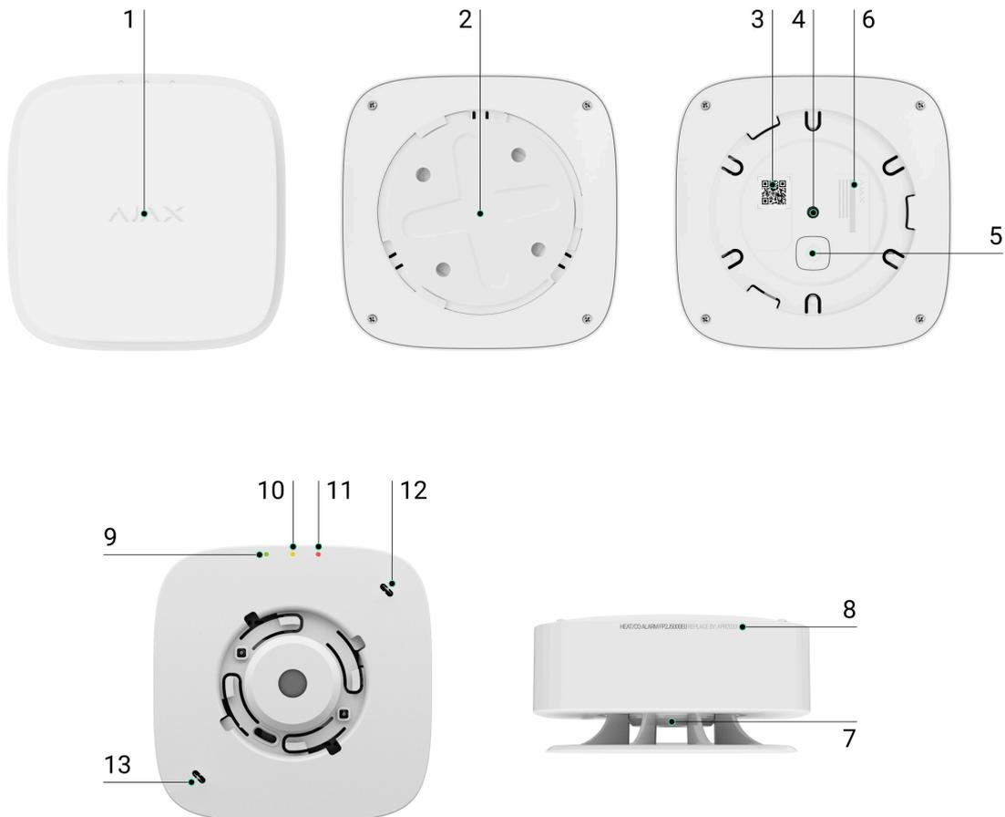
1. Detector front panel with Test/Mute button. To activate the button, press the center of the panel.
