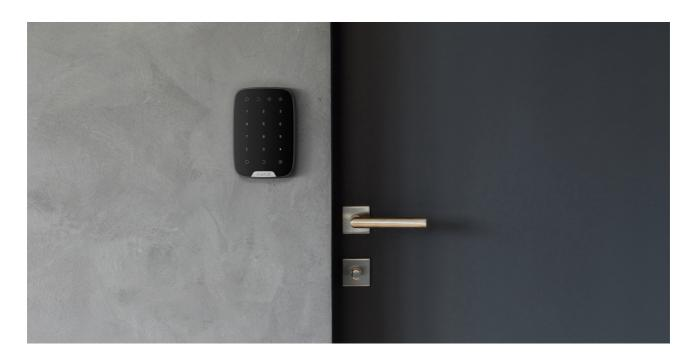
The location of the device depends on its remoteness from the hub, and obstacles hindering the radio signal transmission: walls, floors, large objects inside the room.
