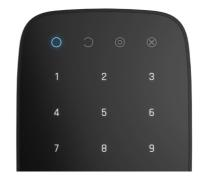
When touching KeyPad, it wakes up highlighting the keyboard and indicating the security mode: Armed, Disarmed, or Night Mode. The security mode is always actual, regardless of the control device that was used to change it (the key fob or app).
