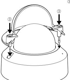
③ Temporarily secure the unit to the enclosure and rotate the long enclosure fixing screw attached to this product clockwise to penetrate the enclosure of the camera.
