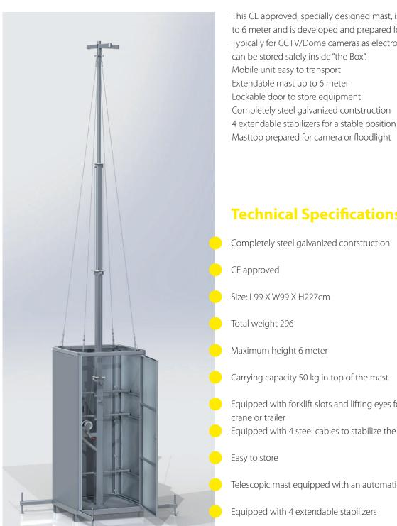
This CE approved, specially designed mast, is extendable to 6 meter and is developed and prepared for all sort of purposes. Typically for CCTV/Dome cameras as electronics equipment can be stored safely inside "the Box". Mobile unit easy to transport Extendable mast up to 6 meter Lockable door to store equipment Completely steel galvanized contstruction
