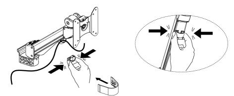
Unattach the small cable collector and route the cables through. Once satisfied, re-attach the collector back into place, and cover the bottom bracket.
