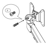
Slide the monitor (with VESA plate) onto the arm and make sure it "clicks" securely into position.
