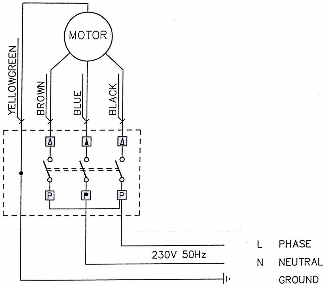
OBS! The wiring diagram above is valid for one motor. When connecting several motors these may not be connected in parallel to the above mentioned switch, but have to be connected to a relaybox. Please require special diagram.
