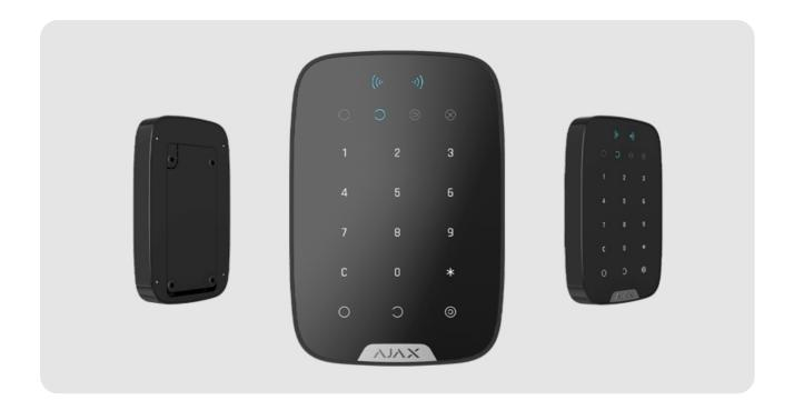
**KeyPad Plus** is a wireless touch keypad for managing the Ajax system with encrypted contactless cards and key fobs. Designed for indoor installation. Supports "silent alarm" when entering the **duress code**.
