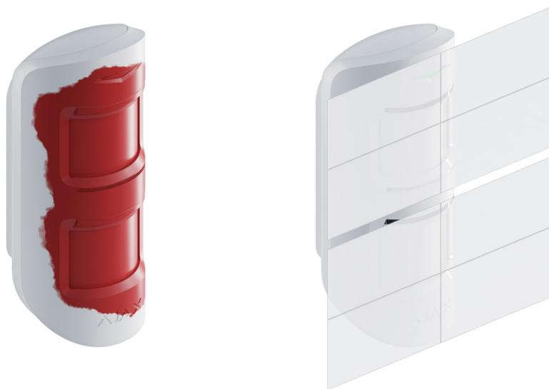
**Masking** is an attempt to block the view of the detector by painting over it, covering it, placing an obstacle in front of the detector's lens, or otherwise.
