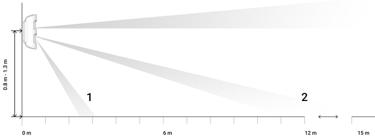
The direction of the lower beam of the detector's IR sensor with a given minimum (1) and maximum (2) detection distance
