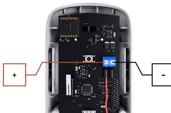
9. Connect the other end of the cable to the power source following the polarity. The power supply must be de-energized at the time of connection.
