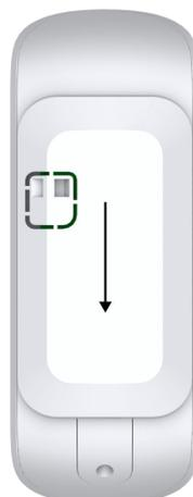
2. Unscrew the screws and carefully remove the rear of the detector enclosure.
