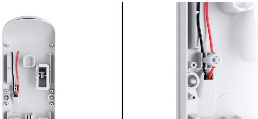
7. Prepare wires for connection. The ends of the wires that will be inserted into the terminals should be be tinned or crimped with special tips. This will ensure a reliable connection.
