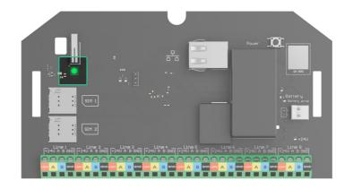
The hub LED has a list of indications showing the system state or events occurring. Hub Hybrid can light up red, white, purple, yellow, blue, or green, depending on the state.
