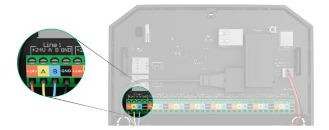
Hub Hybrid (2G) / (4G) has 8 Fibra lines. Numbers from 1 to 8 are indicated on the control panel board.
