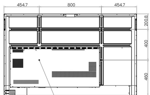
SCREW THREAD DEPTH : 4-M8x25mm
