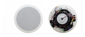
The Galil 8CO is a pair of twoway, openback, 8 speakers designed for mounting in the ceiling. The speakers feature a multitap power transformer for selecting 8 or 70V/100V power settings suitable for array installation
