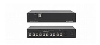
The VA-102P5 is a 10-output power supply that powers 5V DC powered devices. The VA-102P5 can supply a maximum of 1.8A of current to each of ten devices for a total of 18A. The power supply is especially useful in high-population installations for saving space and eliminating a large number of 5V DC power adapters. The MD model is suitable for medical applications.
