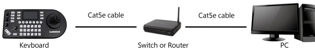
2. To connect directly through network cable, the IP address of the keyboard and PC should be changed to set at the same network segment
