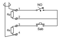
MK440 with built in resistors Rp & Rs Loop A = End of line monitoring using two resistors Loop B = Resistor Rp enables more contacts to be added to the loop.
