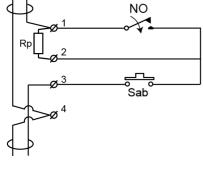
MK440 with two resistors mounted in the terminals for an end of line contact when only one contact used in the loop.
