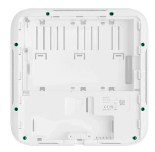
**7.** Slide the latches and carefully remove both boards, keeping them in the same plane and not disconnecting them. There are connectors between boards; do not break them.
