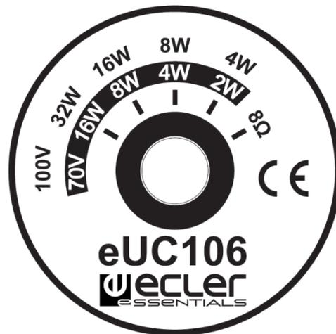
**eUC106 is supplied with the switch in the 70V / 100V position. If you accidentally connect the system to a low impedance 8Ω line, it will not harm the speaker, but the speaker will perform below its real performance level. If the speaker is in the 8Ω position and is accidentally connected to a 70V / 100V line, it will be seriously damaged.**
