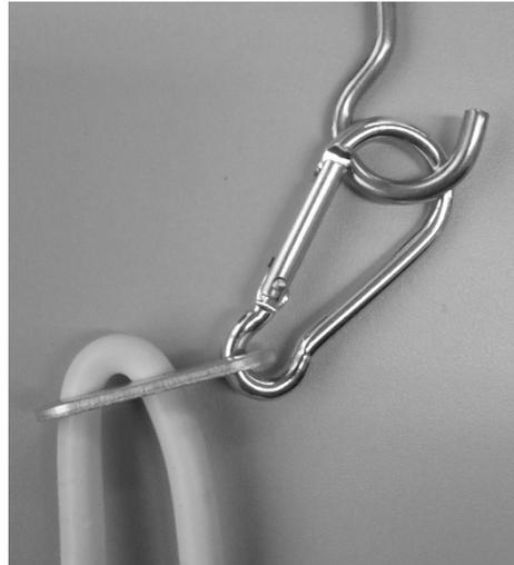
4. Take the safety steel wire from loudspeaker line cable and install it in the clamp as shown in the picture.
