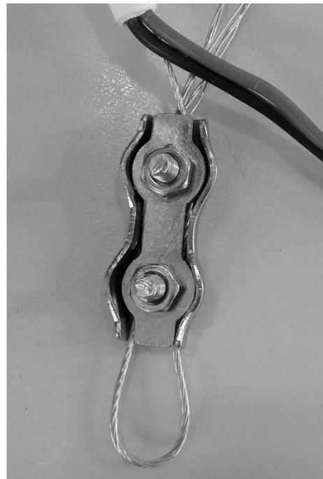
5. In order to make the installation totally secure, introduce safety cable in the eye bolt too.
