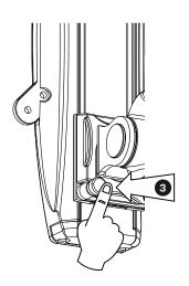
Insert the VESA (with LCD display on already) into the arm and press it down. Then secure fixing lump on VESA with knob. (As figure down step 1. 2.3)
