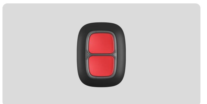
**DoubleButton** is a wireless hold-up device with advanced protection against accidental presses. The device communicates with a hub via the encrypted **Jeweller** radio protocol and compatible only with Ajax system. The line-of-sight communication range is up to 1300 meters. DoubleButton operates from the pre-installed battery up to 5 years.
